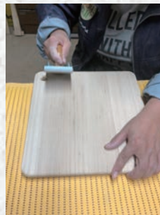
2. Sand the surface with 3 different types of sandpaper.
