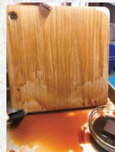
3. Coat the board with the finish extracted from persimmons
