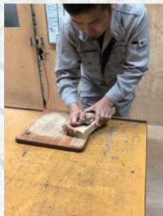
1. Sand the surface with the wood planer.
